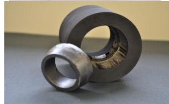
TaC Sub-scale Nozzle and Graphite Die
