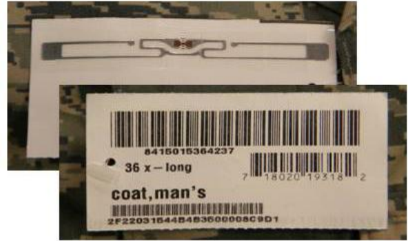
Example of Passive RFID tag on Military Clothing
