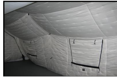
Non-woven Insulation Liner hung within a TEMPER AS
