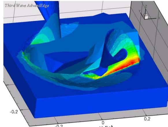
*Simulation of the Drilling Process – Stress State Shown with Red being Highest Stress (Drill Removed)*
