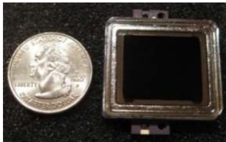
Low Light Level Sensor utilized on vision systems for Apache Helicopter
